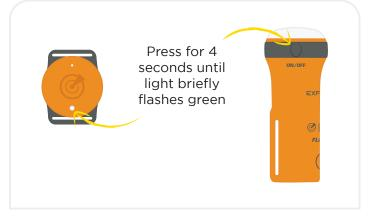
**4.** Switch on 1 x OLAS Tag (or switch on OLAS within the OLAS Float-On).
