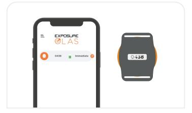
**5.** Check that the tag displayed on the app screen has the same ID number as the tag you are testing with. The tags ID number can be found on the underside of the tag.
