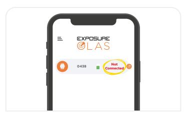
**8.** You may see the tag turn red on the app screen indicating that it has lost signal. If signal is lost for longer than 6 seconds an alarm will sound.
