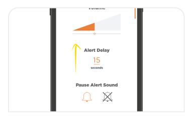
**4.** Adjust the Alert Delay to 15 seconds. This means if the connection between the tag and the mobile device is broken for longer than 15 seconds the alarm will sound.
