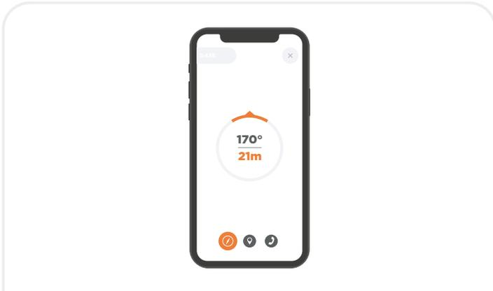
**15.** The 'Searching' screen will change to an arrow pointing back to the 'Point of loss'. It is important to note the arrow DOES NOT track the tag, it points back to the stored GPS location where the alarm occurred, (Note: the accuracy of your GPS can vary depending on your mobile device.)
