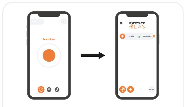
**18.** The Alarm screen will be automatically cancelled when the signal is found again, reverting to the standby home screen.
