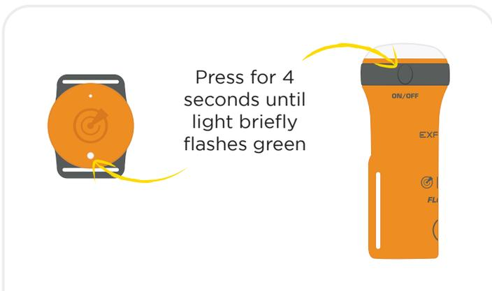
**17.** Switch the OLAS transmitter back on. On an OLAS tag press the button for 4 seconds, you will see a green flash. On the OLAS Float-On press the button for 4 seconds and you will see the lens illuminate green, stop pressing the button and it will start transmitting OLAS.
