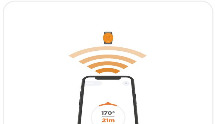
**16.** Follow the arrow towards the 'Point of loss'. This will be within the same area as the switched off OLAS transmitter. The screen will revert to 'Searching' when back within 20 metres.
