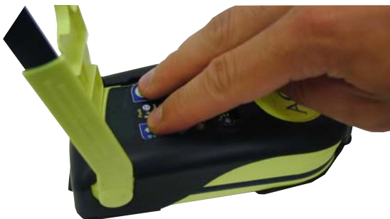
Figure 4 Activation Press both test buttons simultaneously for more than ½ second and no longer than 5 seconds
