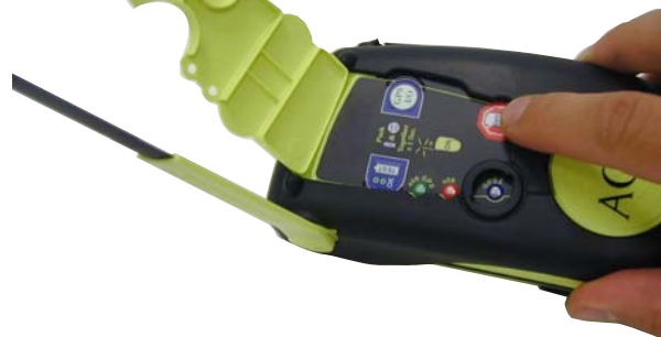
Figure 5 Deactivation Press red OFF button for more than ½ second
